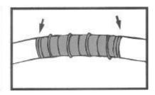
Use abrasive strip to rid hose or cable of loose dirt, grime, and grease in the application area
