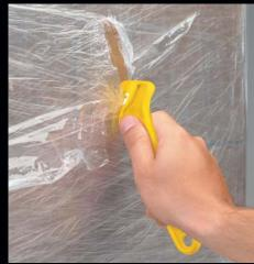
Place thumb on the side grips to firmly guide your cut downward. The tool angle and ultra sharp blade maintain optimum cutting position for cutting shrink wrap from boxes and pallets.
