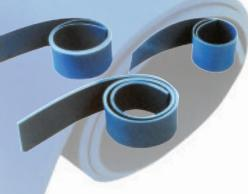
**Detectable sheeting** is available in SEBS rubber in thicknesses of 1.5mm, 3mm and 5mm. The SEBS Rubber is ATEX approved and is static dissipative. Sheeting can be used in a variety of applications from cutting gaskets, o-rings, seals or anywhere there is a chance where a rubber part might break down and cause contamination.
