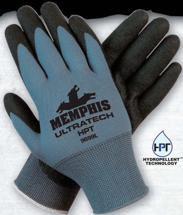
9699 ULTRA TECH® HPT with Hydrepellent Technology™ Sizes: XS-XXL Textured HPT Palm and Fingertips Dipped, 15-Gauge Nylon Shell. CE 4131. Hydrepellent Technology™ process creates a soft, flexible, durable coating that repels liquids and provides a firm wet grip. Hydrepellent Technology™ is a trademark of Midas Safety.
