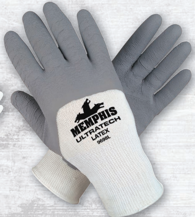
9698 ULTRA TECH® TEXTURED LATEX Sizes: S-XL Textured Latex Over the Knuckle Palm and Fingertips Dipped, 13-Gauge Stretch Nylon Shell. Excellent Grip, Especially for Glass. CE 2131.
